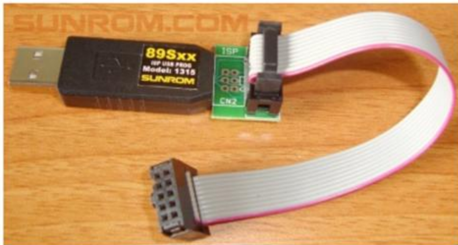
Figure 4.1 89SXX USB ISP Flash Programmer (SPI based)
