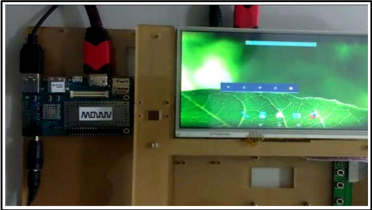
Figure 1.5: Displaying home screen of Dragon board on TFT screen
