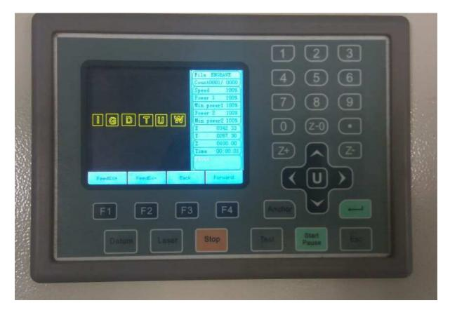
Step10. If you want to PAUSE the process then press the PAUSE Button on computer / on Machine key board and again want to start from there then press START Button. If you want to stop the process then press STOP Button and create New object and Press START button.
