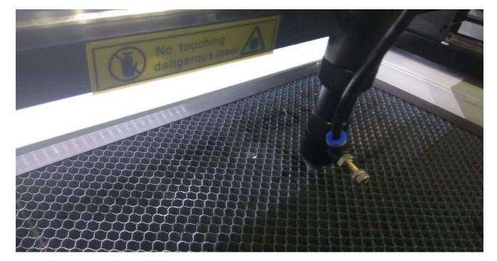
Step8. Click on START after selecting the object and Check on Screen of Machine the object Displayed/detected or not and wait while a Minute. Machine will start to cut the materials. Shown in the fig.
