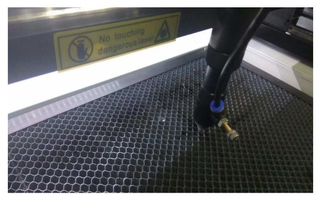
**Step 8.** Check on Screen of Machine the object Displayed/detected or not and wait while a Minute. Machine will start to Engrave the materials. Shown in the fig.
