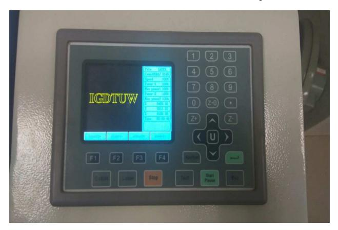
Step10. If you want to PAUSE the process then press the PAUSE Button on computer / on Machine key board and again want to start from there then press START Button.
