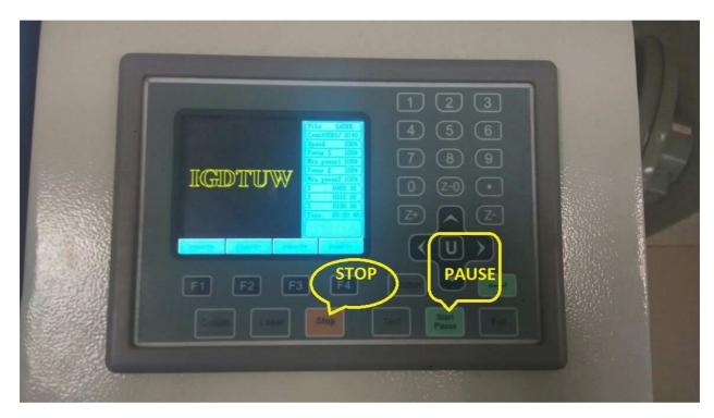
**Step11.** If you want to stop the process then press **STOP** Button and create New object and Press **START** button.
